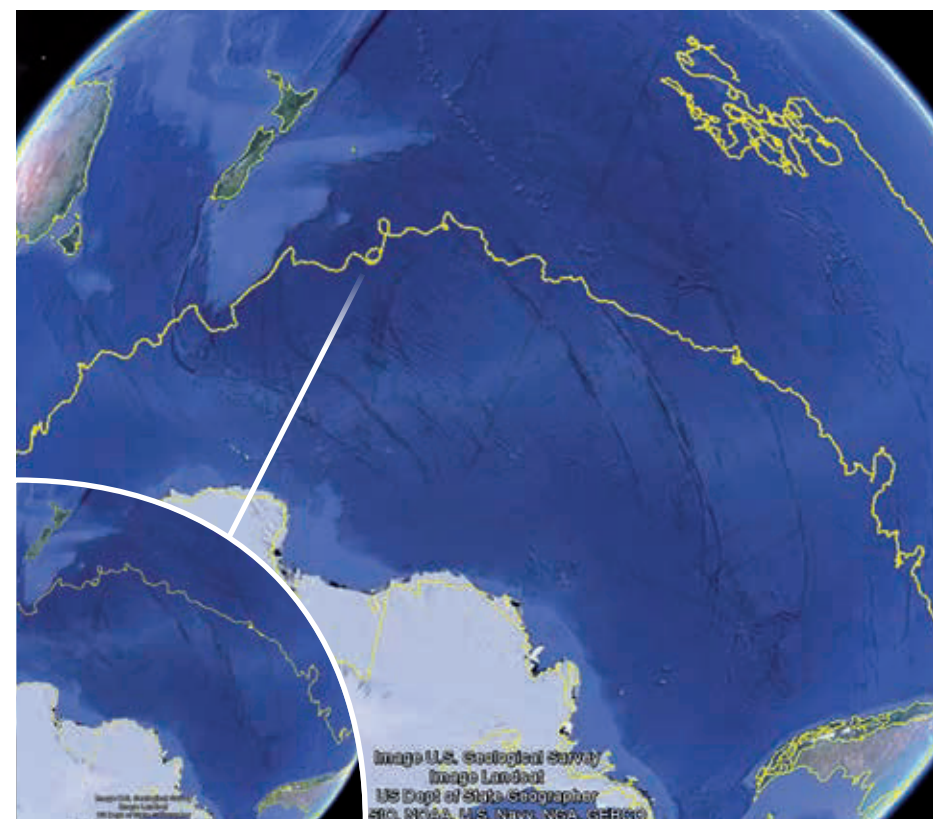
Figure 2. SVP-B buoy (WMO No. 56531, Argos PTT 67381) was deployed on 2 December 2006. The meteorological sensors failed after 954 days of operation on 12 July 2009, but the buoy continued to send position information via the Argos system until 2 August 2014, for a total of 2,800 days.
